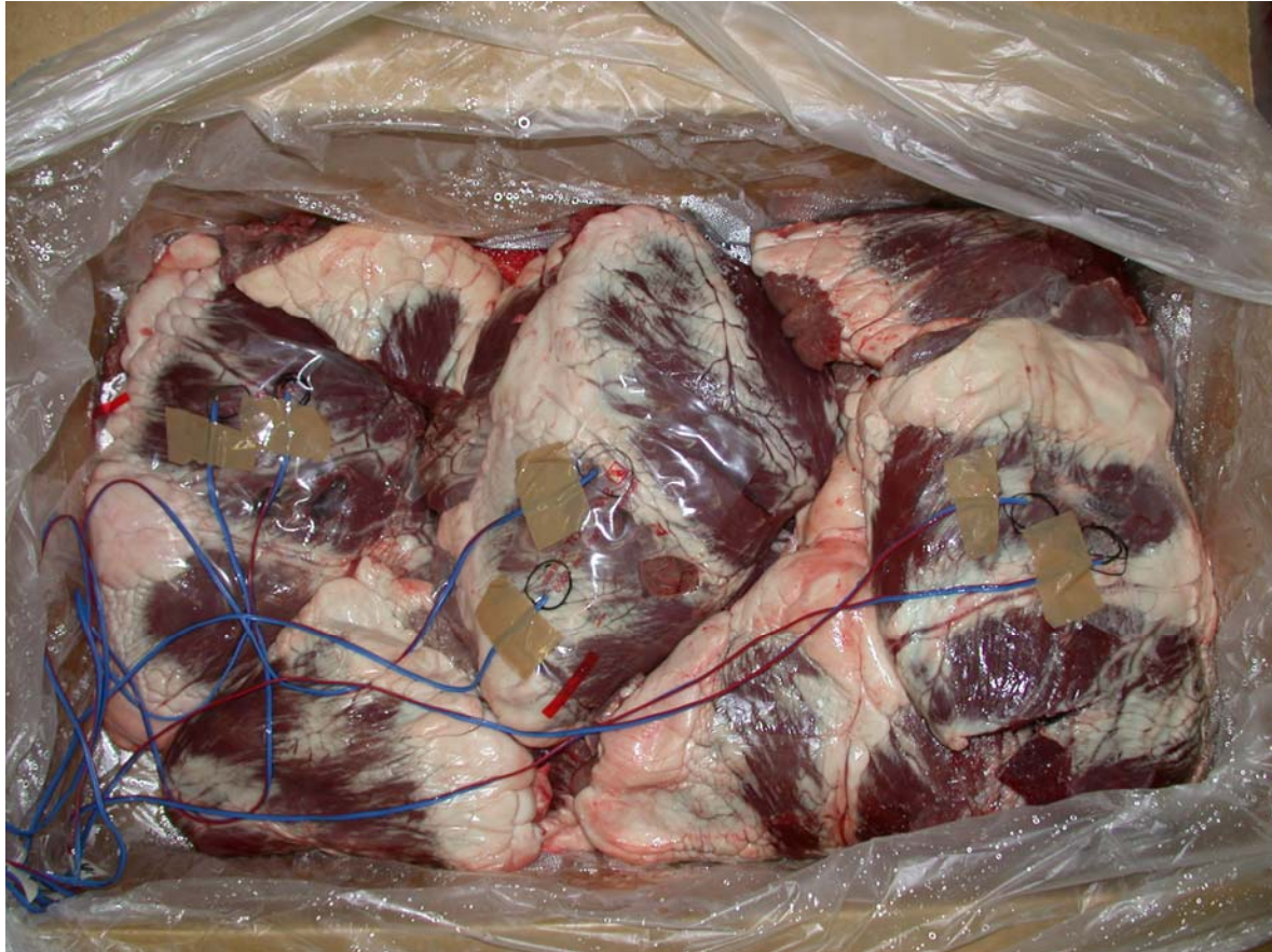
Figure 2: Thermocouples taped to the surface of beef hearts
